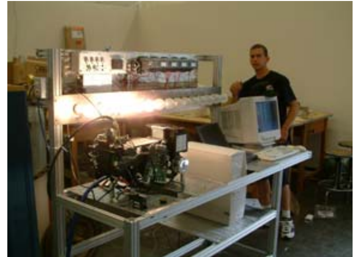
An OREC student tests a 1.2 KW hydrogen-powered fuel cell.
